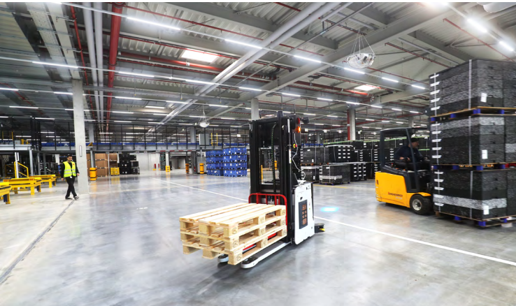
Pallet transport at the new logistics center in Dettingen/Erms is carried out by 15 driverless and battery-operated transport systems.
