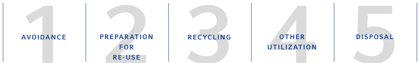
German Closed Cycle Management and Waste Act: Waste hierarchy according to Section 6.
