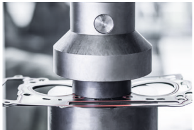
Servo-hydraulic testing facilities for durability tests
