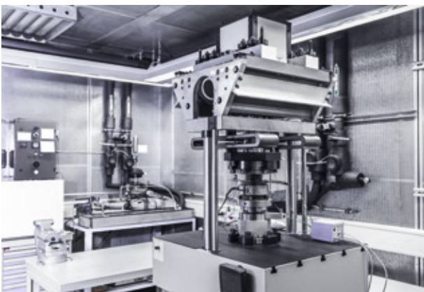
Testing of high-frequency resonance vibrations
